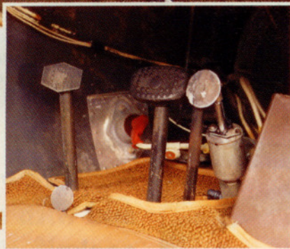
"Four on the floor" in this case refers to the pedals (right). Two rudder pedals control the single rudder—a single pedal is used for braking; the smallest pedal engages the starter.
